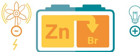
When electricity is stored, it reacts with the zinc bromide solution, forming bromine on the battery electrodes and electroplating the zinc.
