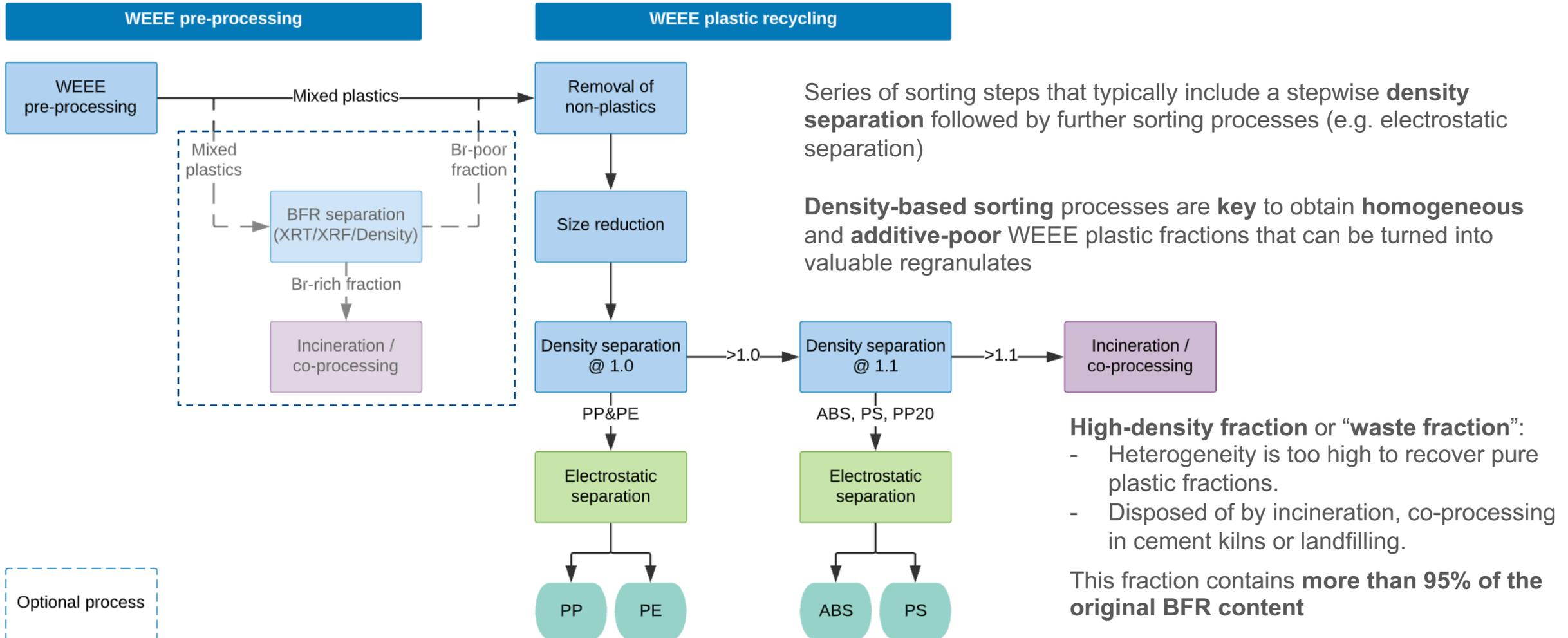
**Target polymers:** pure, additive-poor fractions turned into recycled plastics for the manufacture of new products
